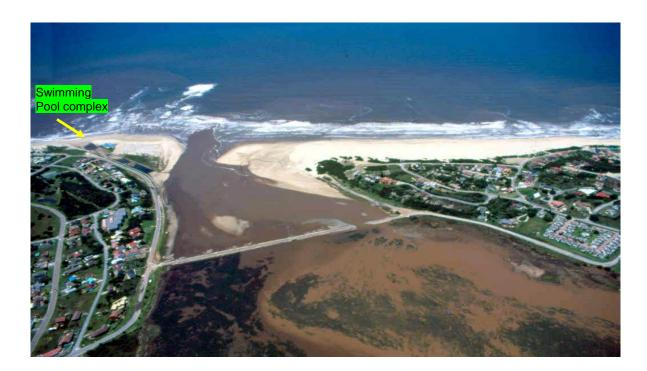
Plate 2 At the time of this photograph (~mid 1980's), the original rubble causeway had been breached and floodwaters eroded a relatively deep and wide channel. The photograph also shows a plume of discoloured estuarine water radiating from the mouth – refer to Figure 5 (Photograph from T Wooldridge).
