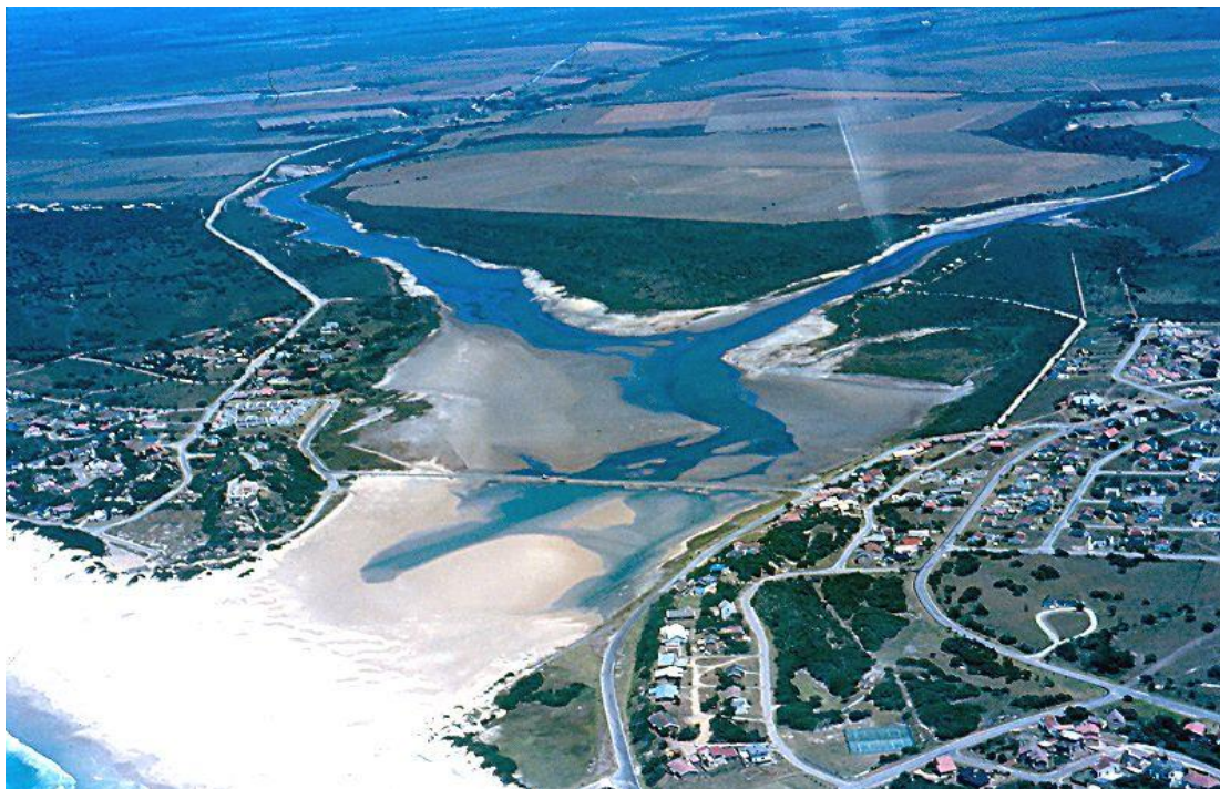
Plate 3 After the construction of the causeway, the Seekoei Estuary was split in to two separate units that essentially blocked tidal flow from reaching up-estuary. More recently, alterations were done to improve the connectivity between the two water bodies. Although it was originally predicted that the upper lagoon would become fresh (Esterhuysen 1982), water abstraction from the catchment has become excessive and the estuary now receives a much-reduced supply – refer Sections 6.7 – 6.8. Occasional floods are also important to remove accumulated sediment, but the barrier effect caused by the causeway reduces scouring. These floods are an important part of a natural cycle in that they also remove large quantities of marine sand that accumulates through tidal transport, overtopping of the sandbar and aeolian transport. Note the extensive area of farming activity north of the Seekoei River Nature Reserve and surrounding the two tributaries (Photograph; T Wooldridge).
